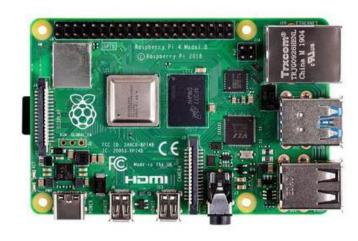
The system will be equipped with 1 raspberry PI V4 (pic 2), This will be the brain of the system and will be able to livestream the video obtained by a raspberry Pi Camera installed in the central dome window. Will also be equipped with 1 arduino uno responsible for the sensors
