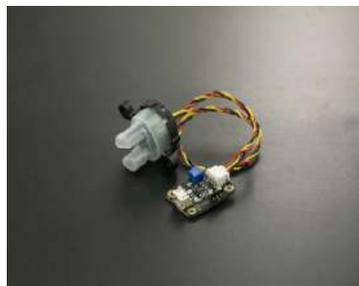
“The turbidity sensor detects water quality by measuring the level of turbidity. It is able to detect suspended particles in water by measuring the light transmittance and scattering rate which changes with the amount of total suspended solids (TSS) in water. As the TSS increases, the liquid turbidity level increases. This sensor has both analog and digital signal output modes. You can select the mode according to the MCU as the threshold is adjustable in digital signal mode. Turbidity
