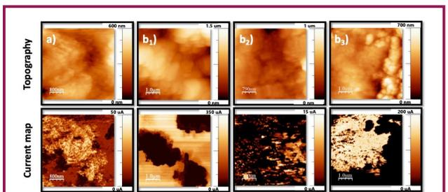
Fig. 4 – Surface topographic and current maps (+0.5 V) obtained by AFM for the anode samples: a) Cell "A"; b1) as prepared Cell "B"; b2) cycle #2 "B"; and b3) cycle #20 Cell "B".
