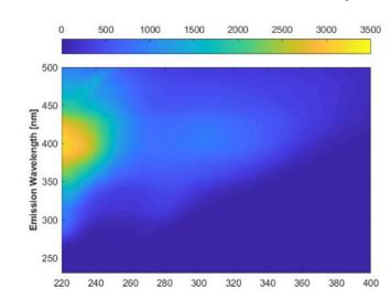
Fig 4: Fluorescence excitation-emission spectrum of aerosol WSOM
