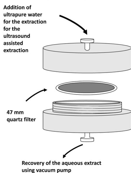
Fig 1: Schematic representation of the proposed Teflon® based apparatus
