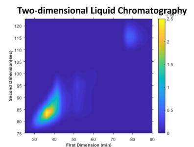
Fig 3: PALC × SEC – FLD (ex: 320 nm; em: 410 nm) chromatogram of aerosol WSOM
