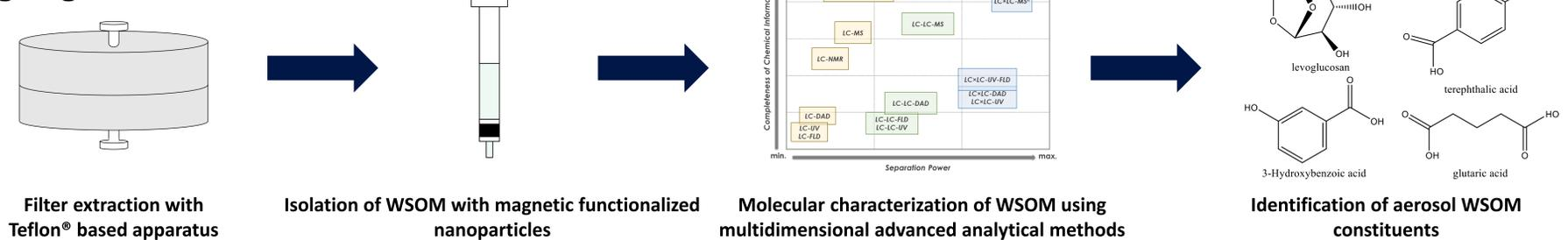
Fig 5: Schematic representation of the methodology for the extraction and isolation of the whole aerosol WSOM
