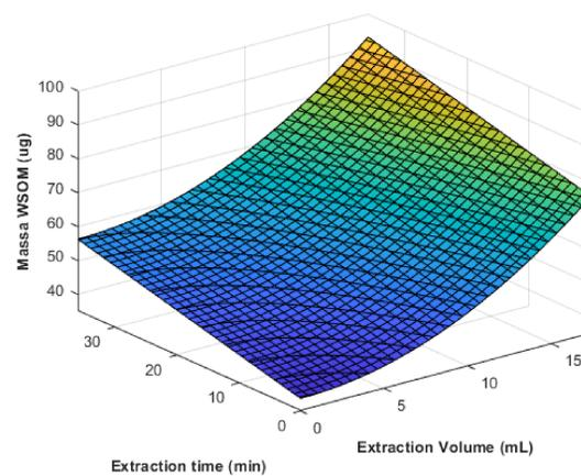
Fig 2: Response surface plot showing the effect of the experimental variables time of extraction and water volume on the amount of WSOM extracted from the urban air particulate matter. The amount of NIST®SRM®1648a is held constant at 2 mg. This model was obtained using a quadratic regression to the uniform experimental design data.
