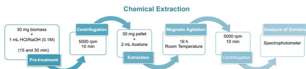
Figure 1. Extraction methodologies.
