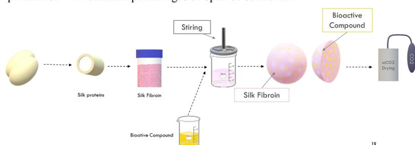
Figure 2 – Silk-based aerogel particles production method.
