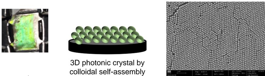
3D photonic crystal by colloidal self-assembly
