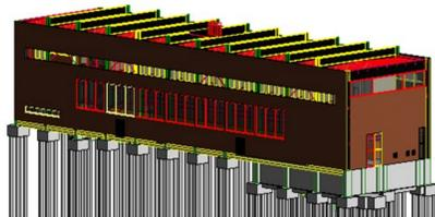
Figure 2 – Visual prioritization of maintenance actions by "color splasher" application to 3D View of the building model.
