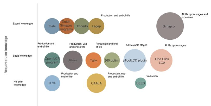
Figure 5 – LCA softwares comparison in terms of required user knowledge and life cycle stages.
