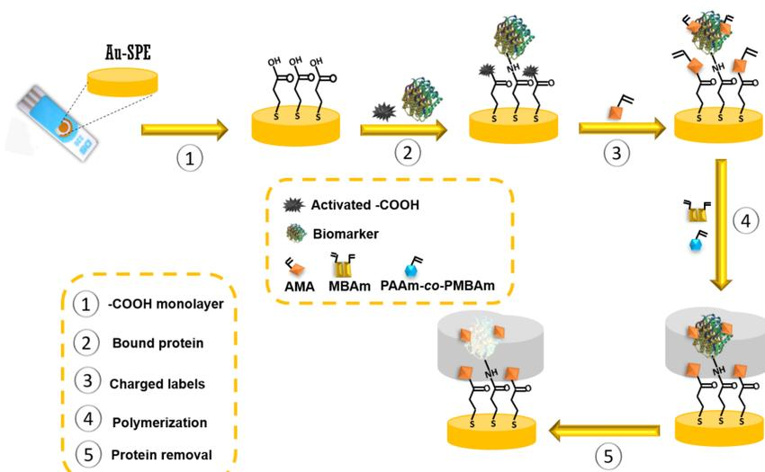
Schematic Illustration of the different steps related to the biosensor device.
