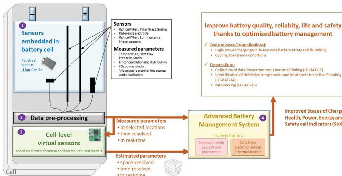
In a nutshell, with INSTABAT the battery will no longer be a black box. It is expected that such a disruptive approach of monitoring/estimating physical parameters and correlating them with battery degradation phenomena will open new horizons to:
