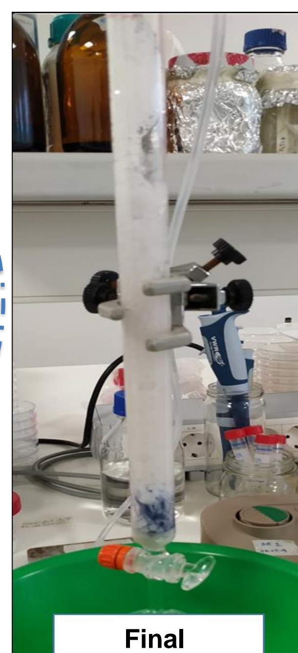
Figure 1 - Decolorization of synthetic effluent Navy Everzol ED (5 g/L) in a preparative column using alginate-calcium capsules with HOMOGST27AB yeast
