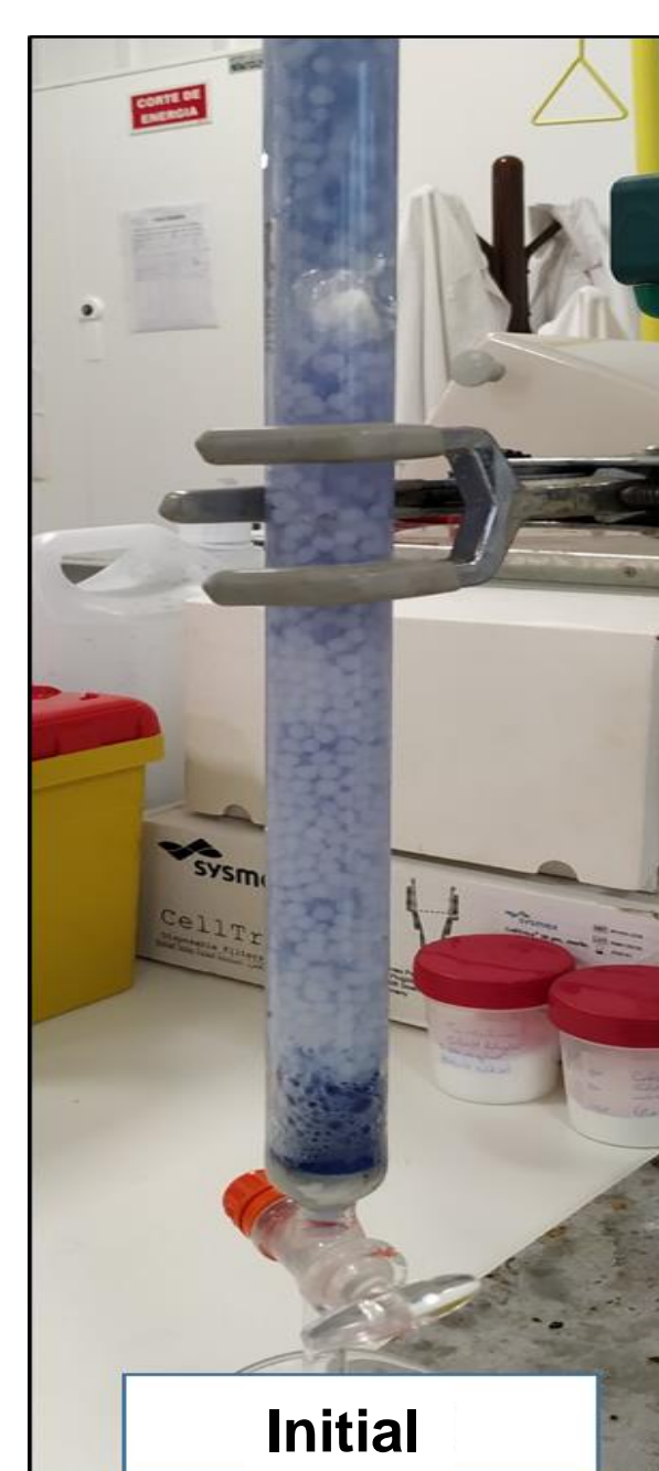
Figure 1 - Decolorization of synthetic effluent Navy Everzol ED (5 g/L) in a preparative column using alginate-calcium capsules with HOMOGST27AB yeast
