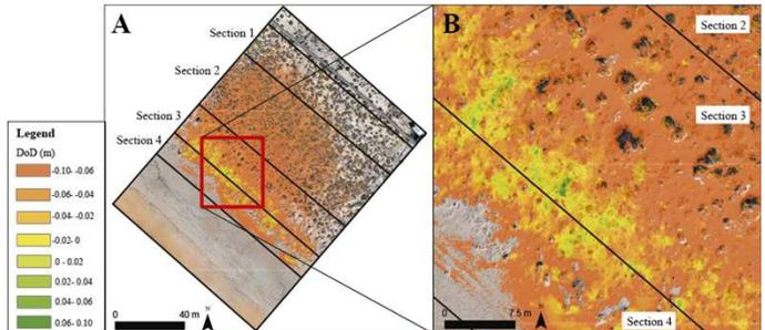
**Figure 3** A Difference of DEM (DoD) over the orthophoto map from October 2020. B detail of DoD.
