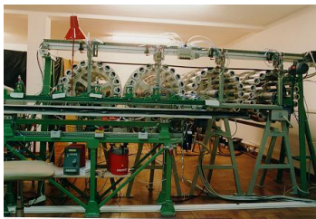
Robot for fiber insertion. 600 000 fibers inserted in Lisbon and later in Coimbra
